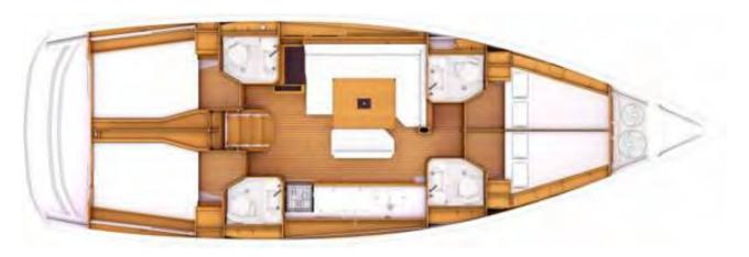
The Sun Odyssey 469 provides a main saloon with each of the four sleeping cabins having its own heads. There is a chart table to port in front of the heads with control panel, GPS and VHF radio and CD/radio player. The main saloon settee and table can convert into an additional large double berth (although this is only suitable for children).
