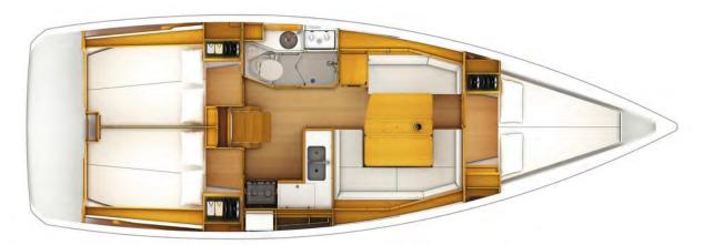
The Sun Odyssey 389 provides a single heads to port, a forepeak cabin with hatch onto the foredeck and two stern cabins. There is a chart table to port in front of the heads with control panel, GPS, DSC VHF radio, EPIRB and CD/radio player.
