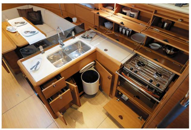
The galley includes a sink, top-entry fridge, twin-burner cooker with grill and plenty of storage both behind the worktop & cooker and below the sink.
