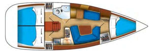
The Sun Odyssey 35 provides a single heads to port, a forepeak cabin with hatch onto the foredeck and two rear cabins. There is a chart table to port in front of the heads with control panel, GPS, DSC VHF radio, EPIRB and CD/radio player.
