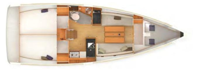
The Sun Odyssey 349 provides a single heads to port, a forepeak cabin with hatch onto the foredeck and one/two stern cabins. There is a chart table to port in front of the galley with control panel, GPS, DSC VHF radio, EPIRB and CD/radio player.
