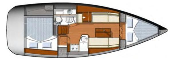
The Sun Odyssey 33i provides a single heads to port, a forepeak cabin with hatch onto the foredeck and one rear cabin. There is a chart table to port in front of the galley with control panel, GPS, DSC VHF radio, EPIRB and CD/radio player.
