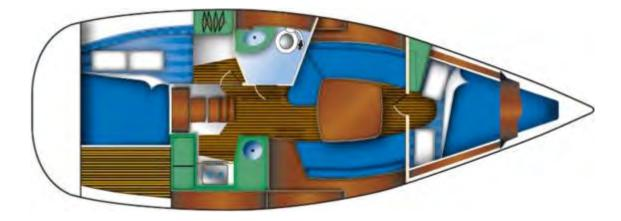
The Sun Odyssey 32i provides a single heads to port, a forepeak cabin with hatch onto the foredeck and one rear cabin. There is a chart table to starboard in front of the galley with control panel, GPS, DSC VHF radio, EPIRB and CD/radio player.
